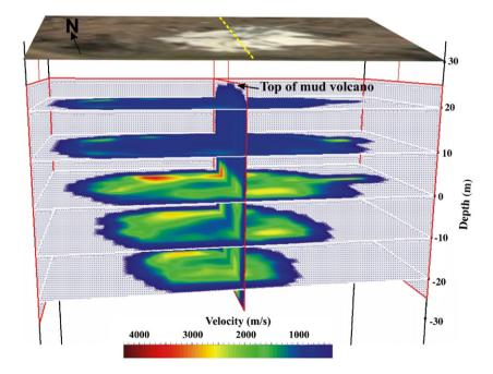
Fig. 7. Depth slices of the velocity model obtained by the inversion of the first breaks. The top of the mud volcano is 22 m.
