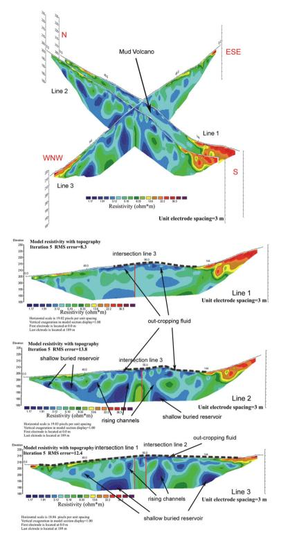
Fig. 10. Result of the tomographic inversion of the geo-electric lines. In the top a 3D view of the lines is shown. The broken grey lines indicate the seismic coverage.
